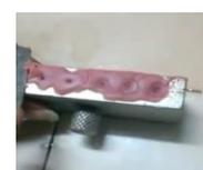
10. Lipstick were removed from mould and prepared lipstick were fitted in lipstick container and used for evaluation.
